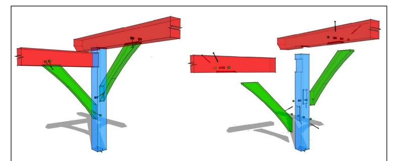
The joint utilizes fully threaded structural screws along with a 3/4" housing. Two screws at each end, one from each side at 45 degrees each way holds everything together. We have found that a 1 1/4" hole allows you to easily install the screws and gives you enough room for the blind pegs that give you that traditional look. We use the Rothoblaas VGZ screws in 7mmx 180mm (7.077") in our plans, kits, and designs.
