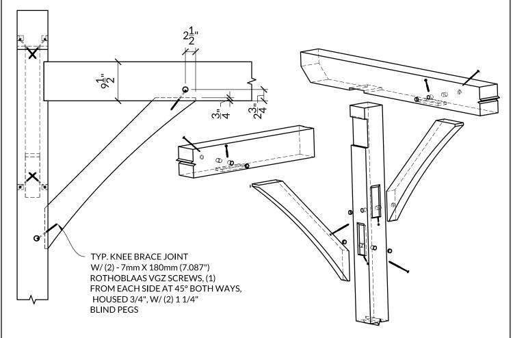
A Post and Beam Knee Brace Connection SCALE: 3/4" = 1'-0"
